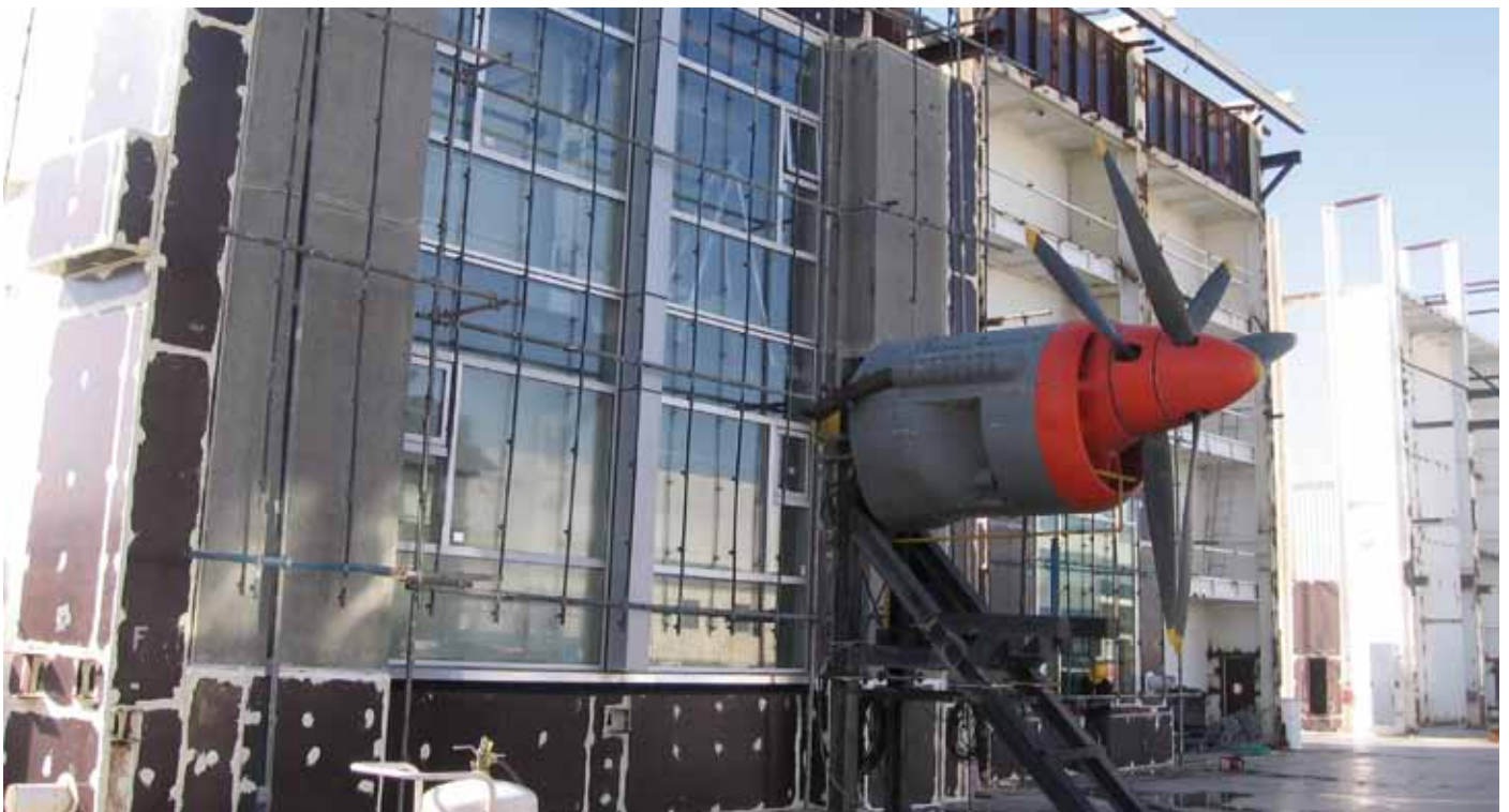
The dynamic water tightness is tested by an aircraft propeller.
